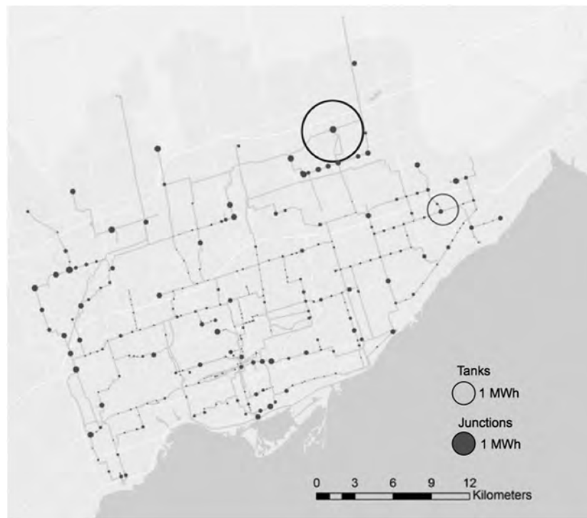
Fig. 13. Map of energy delivered in the Toronto water distribution network during peak demand (8 p.m.) on maximum demand day
