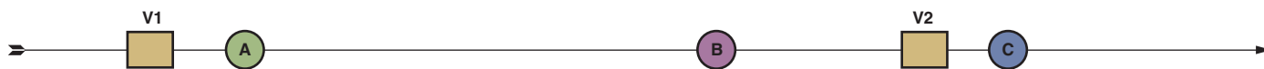
FIGURE 2 Schematic of the pressurized section between two valves (V1, V2) at Sheffield and the location of three pressure sensors (A, B, and C)
